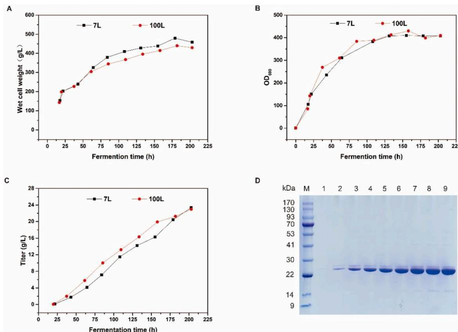
Fig. 4. The time-course of wet cell weight (A), OD value (B), titer (C) and non-reducing SDS-PAGE analysis (D) at 7 L and 100 L scale. M, prestained molecular weight markers; lanes 1–9, 0.5 μL culture supernatants after 0, 18, 42, 66, 90, 114, 138, 162 and 183 h of induction at 100 L scale.
