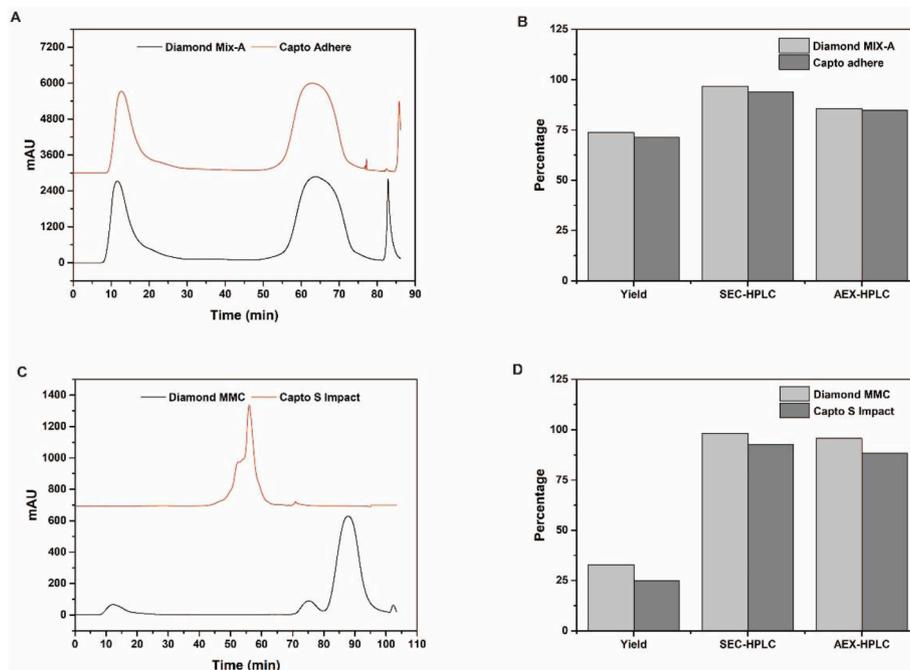
**Fig. 5.** Purification process development of Nb3341. (A) Chromatograms of Diamond Mix-A and Capto Adhere. (B) Yield, SEC-HPLC and AEX-HPLC of Diamond Mix-A and Capto Adhere. (C) Chromatograms of Diamond MMC and Capto S ImpAct. (D) Yield, SEC-HPLC and AEX-HPLC of Diamond MMC and Capto S ImpAct.
